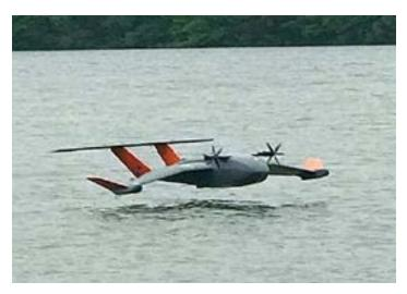
These vehicles start out on the water, but then increase speed and actually take to the air — skimming over the water on a cushion of air.
